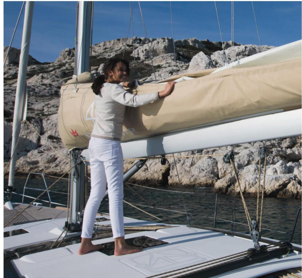
Inclined boom for easy packing
