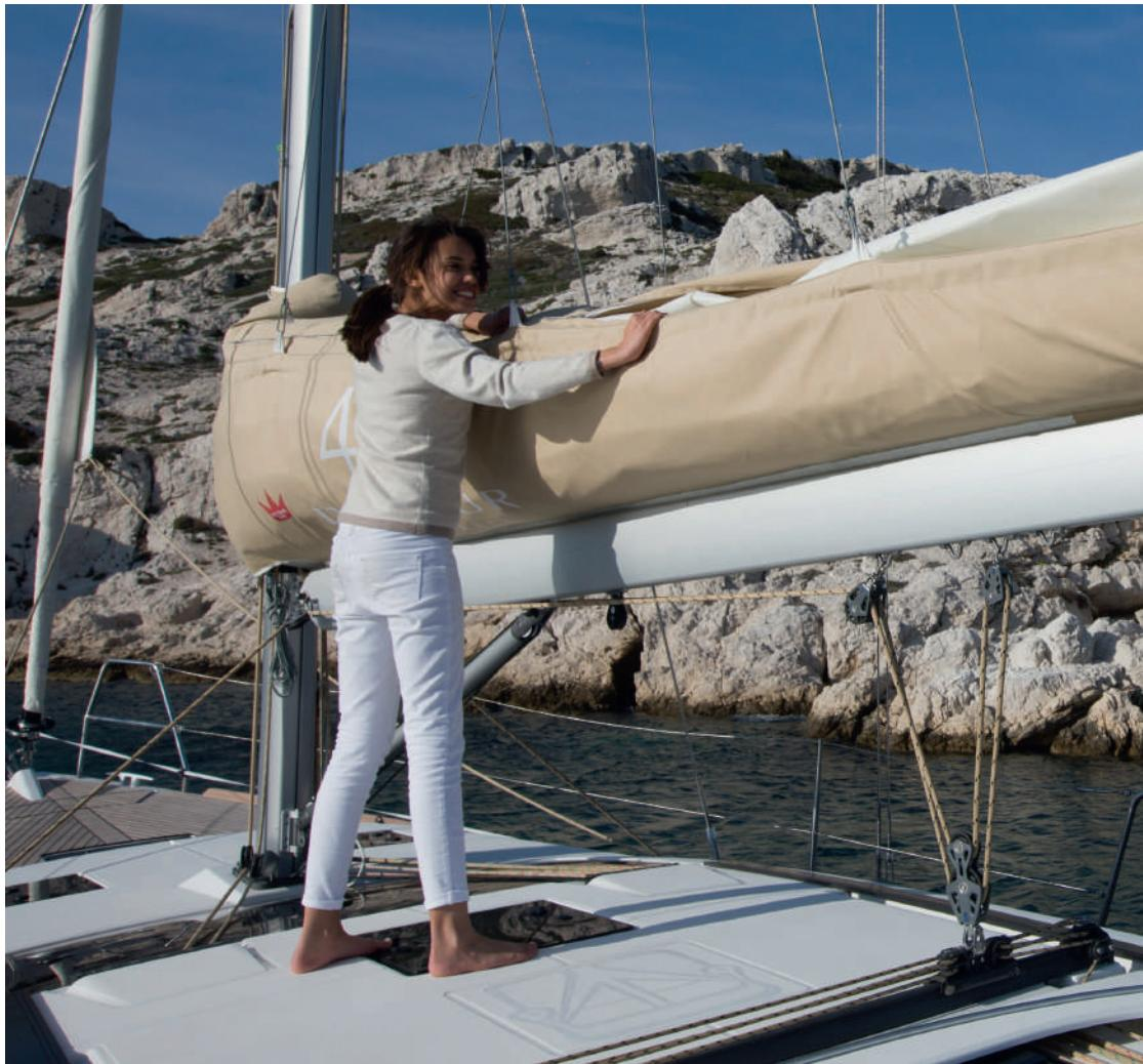
Inclined boom for easy packing
