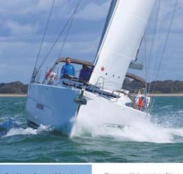
We were unable to experience this as our test boat had in-mast reefing. Both the main and the standard self-tacking jib were in Dacron and from the Envstrom loft in France, the main being without battens since Z-Spars has always advised against them with its in-mast reefing. To get the boat going at its best, you would want to replace the Dacron sails with laminates and/or opt for a conventional mainsail. A taller rig in carbon is an option too.
